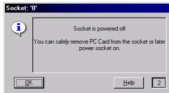
**NOTE:** Removing the SRAM Card without first stopping the device is not recommended. This could cause malfunction in the device that may lead to data lost and/or lost of the SRAM format. In case of lost of format, the Card needs to be reformatted by either the PP1 or 4300 unit.
