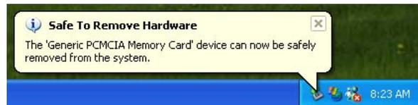
**NOTE:** Removing the SRAM Card without first stopping the device is not recommended. This could cause a malfunction in the device that may lead to data lost and/or lost of the SRAM format. In case of lost of format, the Card needs to be reformatted by either the PP1 or 4300 unit.
