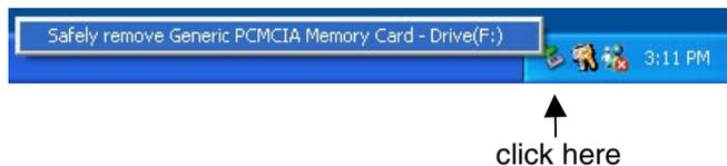
2. The following message will appear on the lower right side of the screen. Now it is safe to remove the **SRAM Card** from the **PCMCIA** slot.
