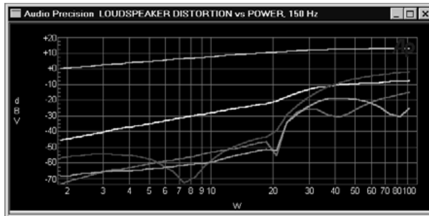
Figure 12-3 Fundamental (top curve), 2nd harmonic, 3rd harmonic, 4th harmonic, and 5th harmonic amplitudes of a loudspeaker as a function of power.
