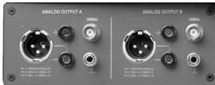
Figure 1-2 Analog Generator (Upper Left) Output Connector Panel
