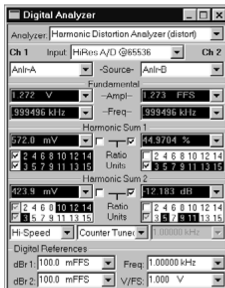
Figure 12-1 Harmonic Distortion Analyzer Panel, Large Form
