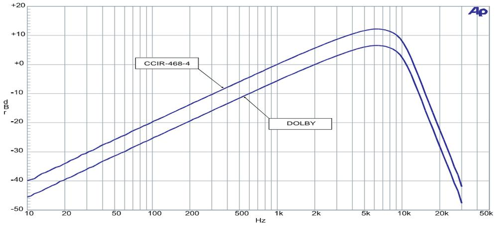
Shape of CCIR Filter - CCIR-468-4 has the 0 dB point at 1 kHz, while the Dolby curve has the 0 dB point at 2 kHz.
