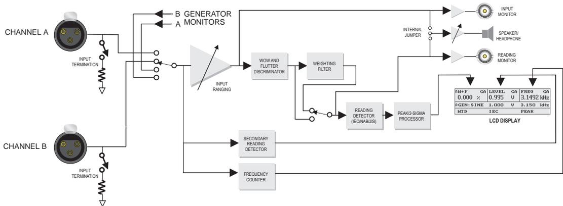
Figure 4-32 Block Diagram of Analog Wow and Flutter Measurement
