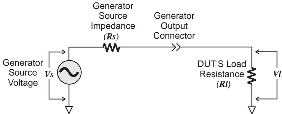
Figure 4-11 Source and Load Impedances
