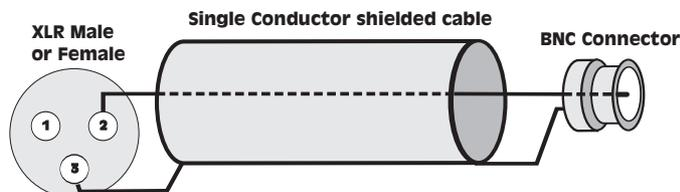
Figure 6-7 Unbalanced Connections Using Single-Conductor Cable
