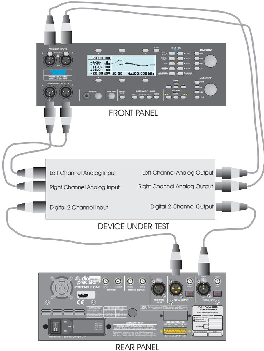
Figure 2-7 Typical Connections to Analog and Digital Device
