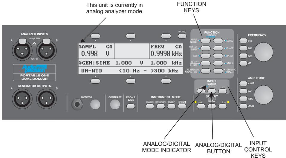
Figure 4-13 Analyzer Control Keys
