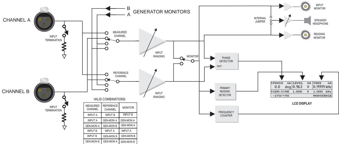
Figure 4-25 Block Diagram of Analog Phase Measurement
