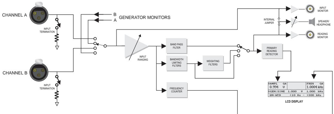
Figure 4-15 Block Diagram of Analog AMPL Measurement
