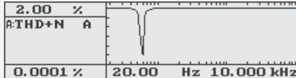
If you see this graph, you should immediately suspect that the THD+N reading is dominated by a significant component at the frequency of the dropout.
