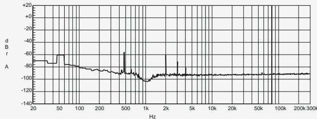
This signal contains contributions from harmonic distortion (at 2 kHz, 3 kHz, and 4 kHz), an interfering tone (at 490 Hz), random noise, and 60 Hz hum. The THD+N measurement includes all of these, and reads 0.229 %.
