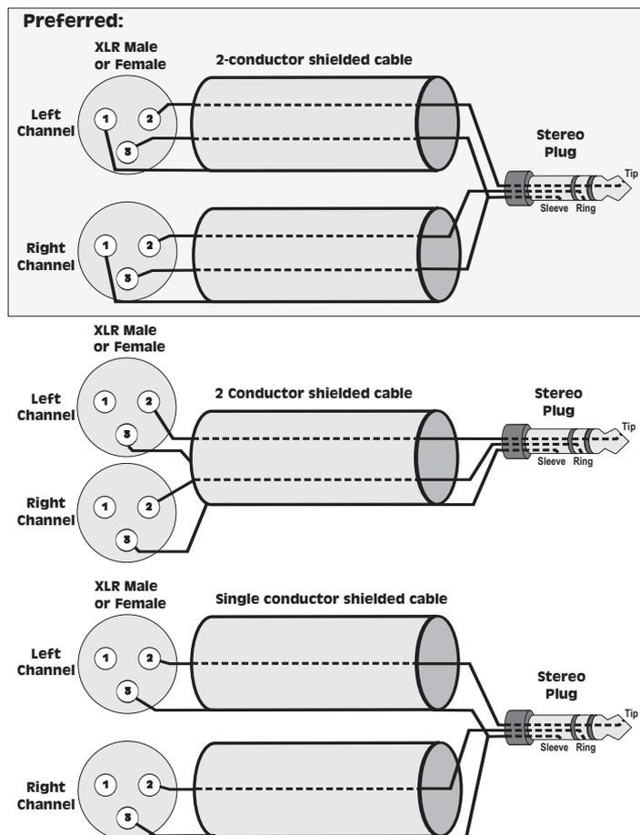
Figure 6-8 Stereo Unbalanced Cable Connections
