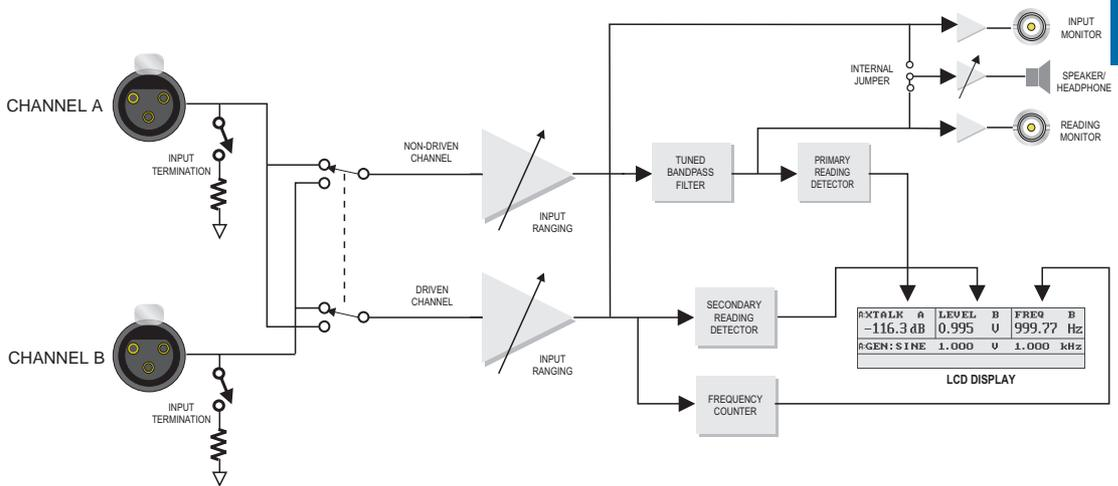
Figure 4-34 Block Diagram of Analog Crosstalk Measurement
