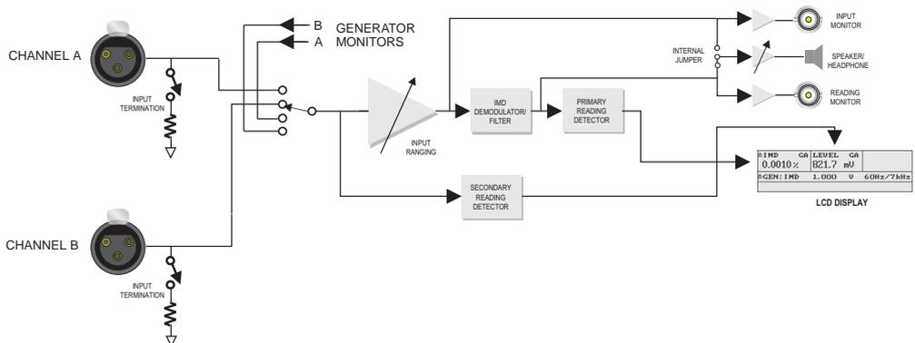
Figure 4-27 Block Diagram of Analog IMD Measurement
