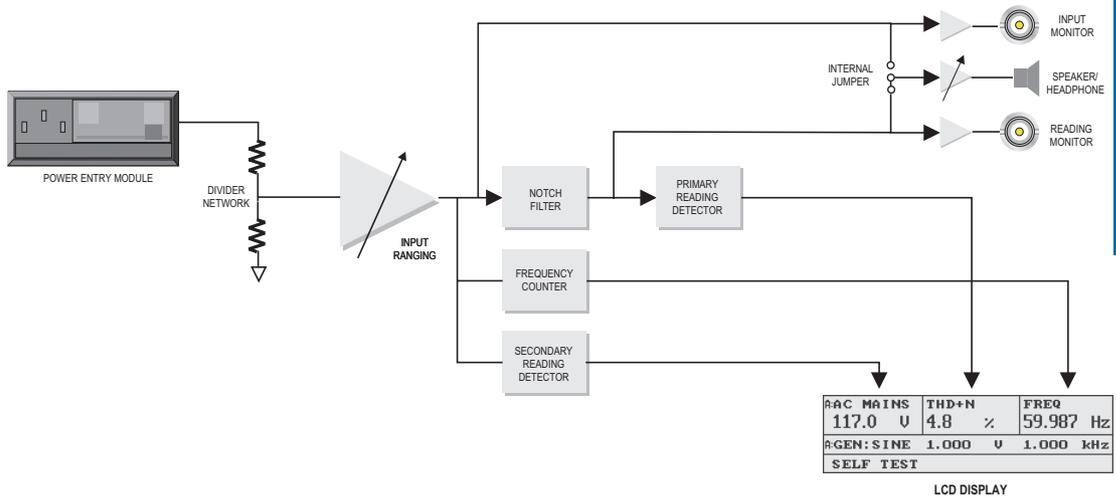
Figure 4-36 Block Diagram of AC Mains Measurement
