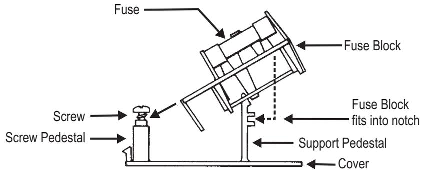
Figure 10-4 Insertion/Removal of Fuse Block
