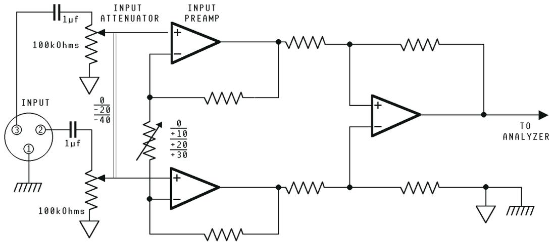
Figure 6-4 Simplified Analog Analyzer Input Circuit
