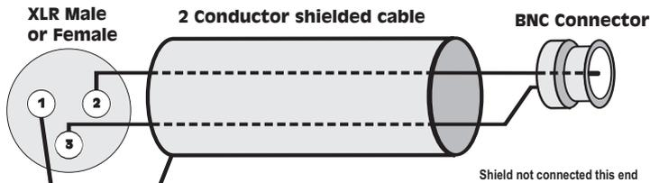
Figure 6-6 Preferred Unbalanced Cable Connections
