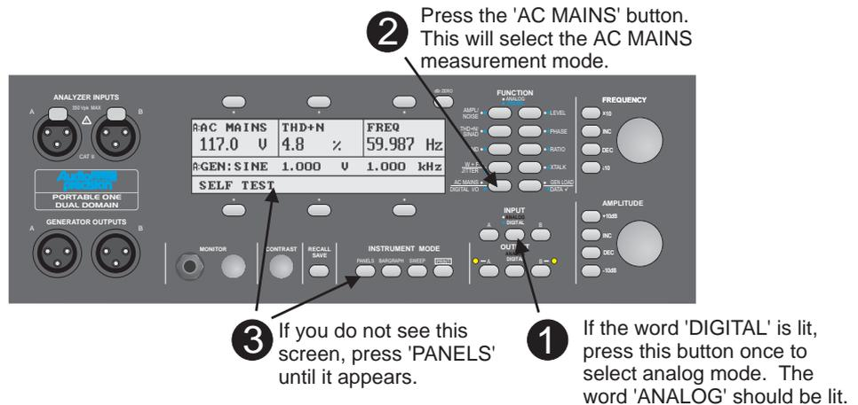
Figure 12-1 Steps to the Main Panel in AC Mains Function
