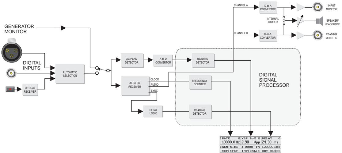
Figure 4-42 Block Diagram of Digital I/O Measurement
