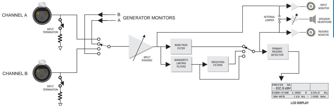
Figure 4-17 Block Diagram of Analog NOISE Measurement
