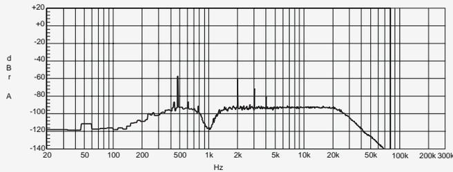
The THD+N still measures 0.185 %. From this, we can determine that (in this particular case) the high-frequency noise did not make a significant contribution to the measurement. It is dominated by the distortion and interference tones.
