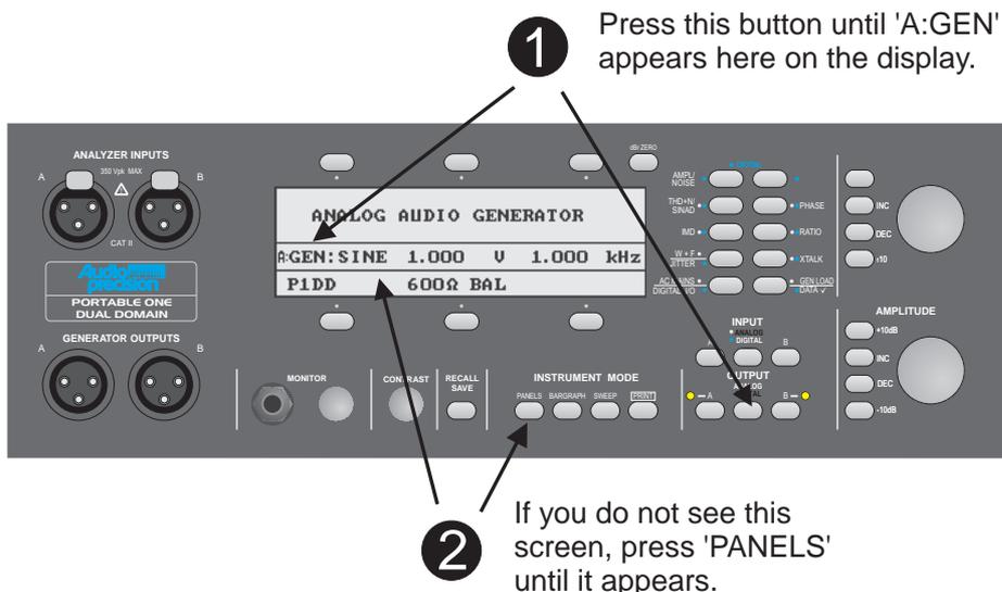
The lower center soft key selects the generator output impedance and configuration. The choices are '40  $\Omega$  UNBAL', '40  $\Omega$  BAL', '150  $\Omega$  BAL' and '600  $\Omega$  BAL'.
