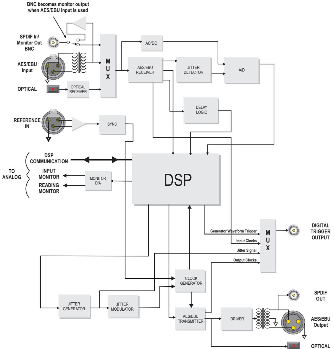
Figure 6-2 Digital Block Diagram
