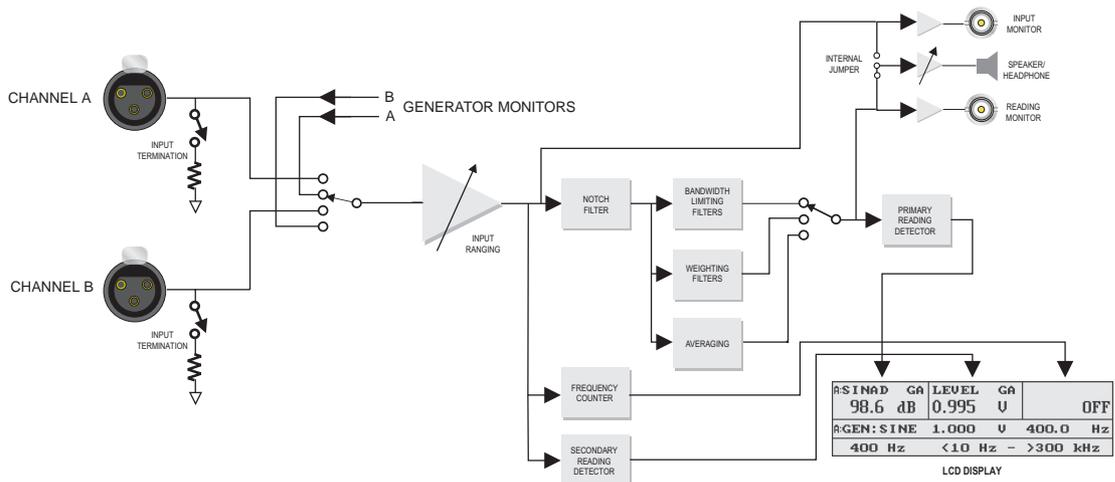
Figure 4-23 Block Diagram of Analog SINAD Measurement
