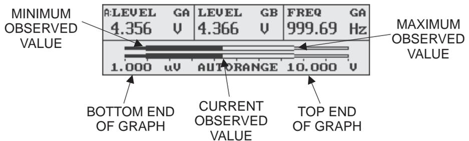
Figure 4-50 Bargraph Screen in Level Function
