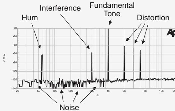
The signal is measured with a voltmeter at this point. The measurement will be dominated by the amplitude of the fundamental tone, since it is at a high amplitude relative to the unwanted signals.
