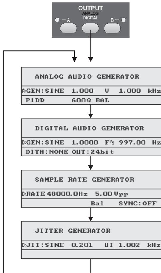
Figure 4-10 Generator Control Modes (Generator Only Panel)
