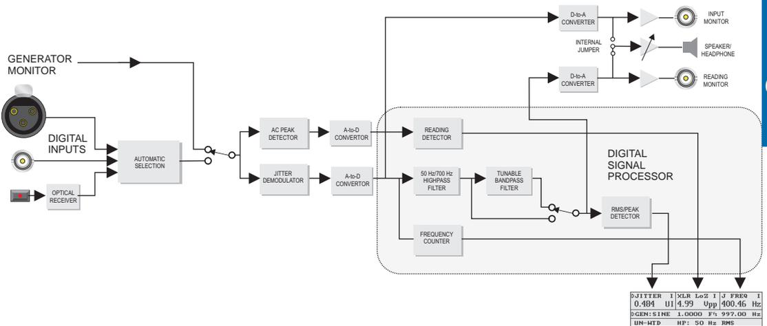
Figure 4-40 Block Diagram of Jitter Measurement
