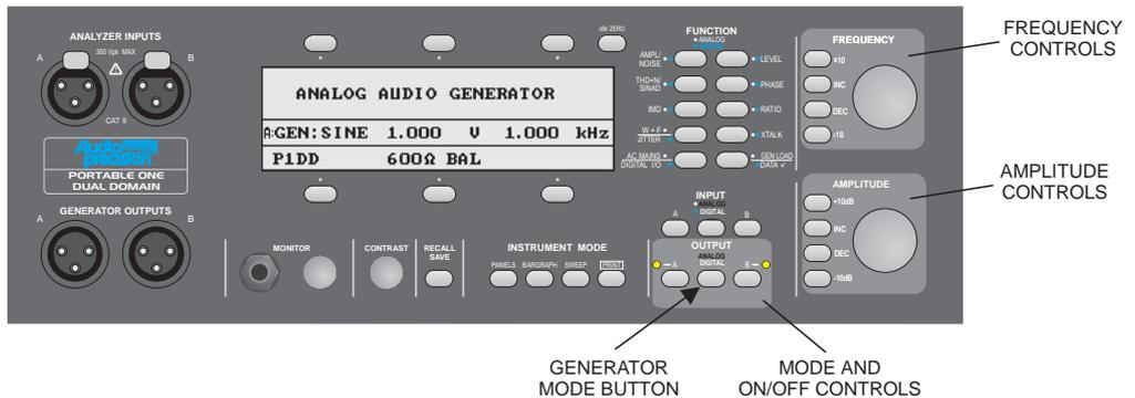
Figure 4-9 Generator Controls
