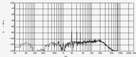
The high-frequency noise has been eliminated, and the measurement is now dominated by the distortion products. The THD+N now measures 0.0390 %, which is precisely the theoretical THD for these distortion products. The contribution of the remaining noise (between 400 Hz and 22 kHz) is negligible.
