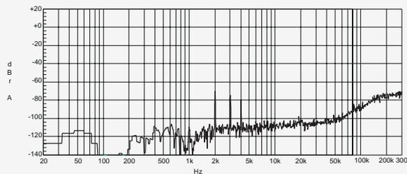
This measurement is dominated by the high-frequency noise, although the distortion products (at 2 kHz, 3 kHz and 4 kHz) are probably contributing. Next, we can invoke the 22 kHz lowpass filter. The spectrum then looks like this:
