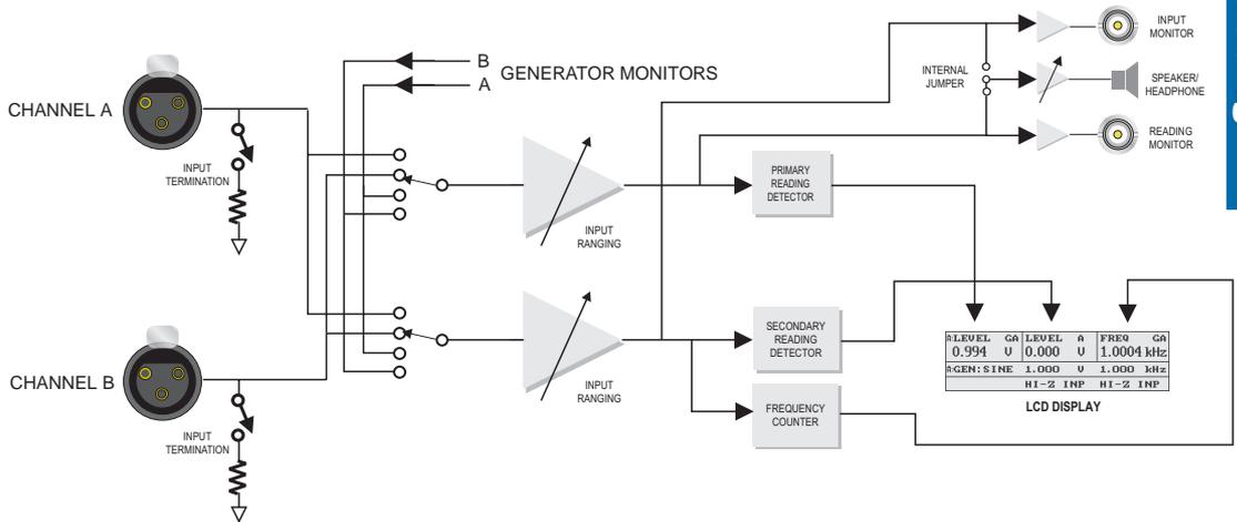
Figure 4-19 Block Diagram of Analog LEVEL Measurement
