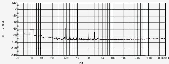
After the bandpass filter eliminates the 1 kHz fundamental tone, we are left with the following:
