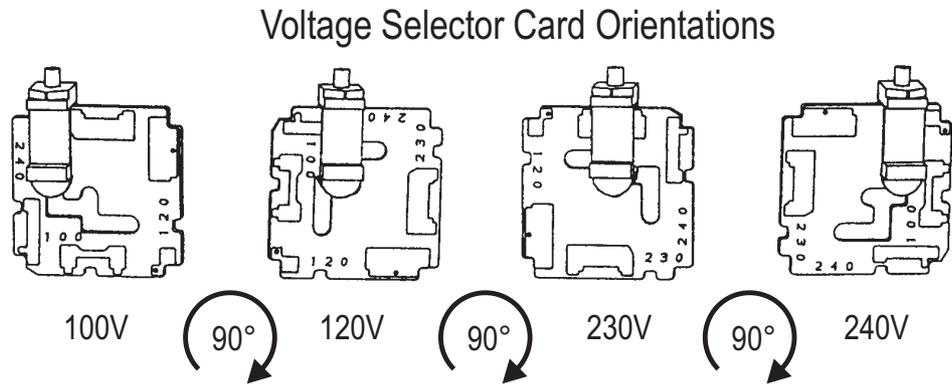
*Figure 10-3 Proper Orientations for Selector Card*
