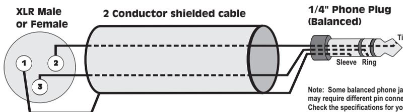
Figure 6-5 Balanced Cable Connections
