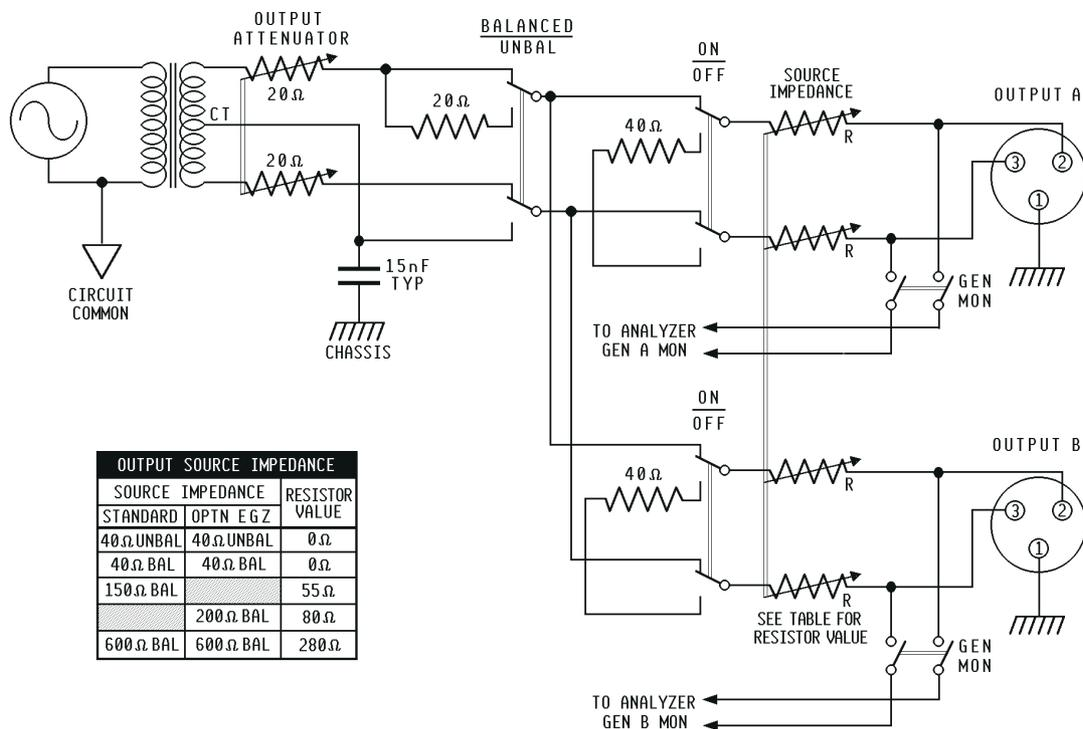
Figure 6-3 Simplified Analog Generator Output Circuit
