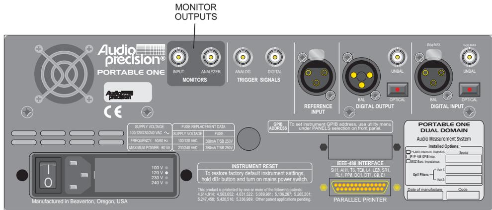
Figure 3-5 Rear Panel with Monitor Outputs Marked
