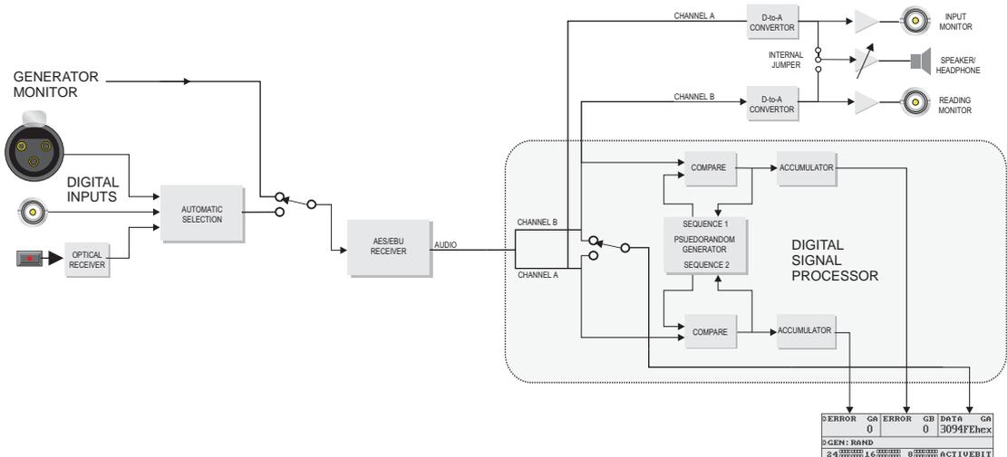
Figure 4-43 Block Diagram of Data Check Measurement
